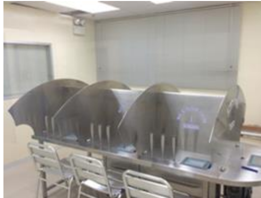
Figure 3: Olfactory Laboratory with Scentroid™ SS600 Olfactometer
